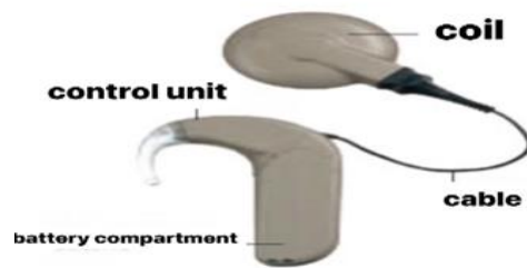
Fig. 2 - External component of the cochlear implant ( https://ascultaviata.ro/wp-content/uploads/2015/06/Sa_intelegem_implantul_cohlear.pdf )
